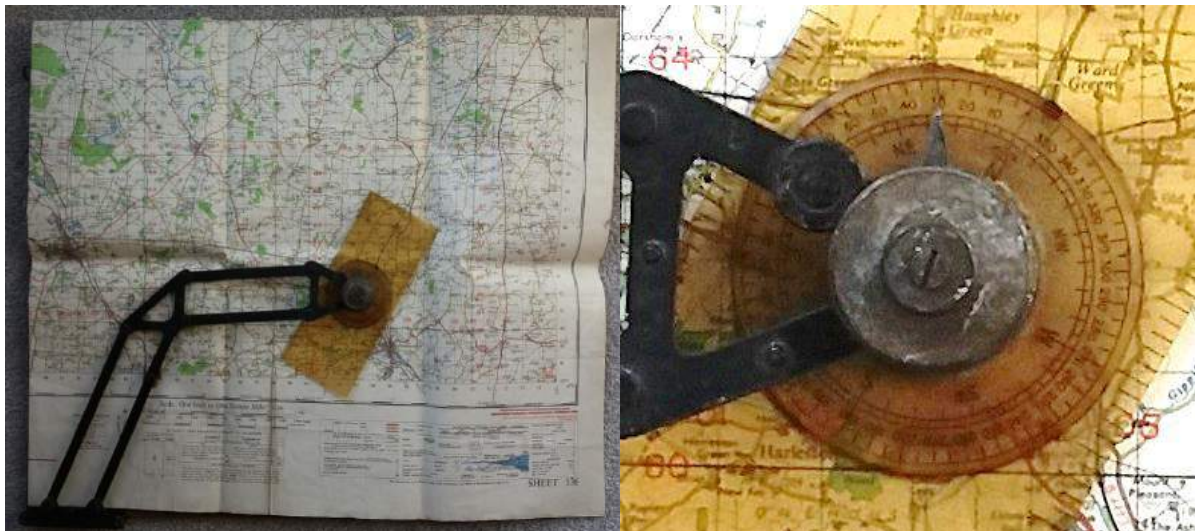
Figure 8.1: Navigator's mapping table with movable arm allowing a course to be plotted and detail of the North pointing arrow (circled) and movable protractor
