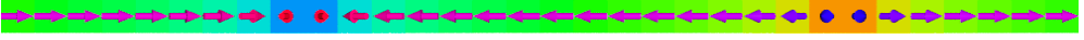
Figure 4.20: Stable 2\pi domain wall in a nanowire. The nanowire is represented by a chain of N = 32 magnetic moments. Arrows indicate orientation of the moments. Periodic boundary conditions are applied along x direction.
