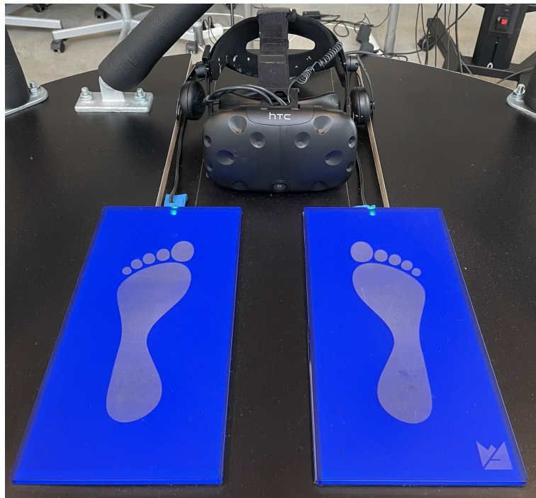
Figure 5.4: Force Plates and VR goggles on the moving platform of BioVRSea
