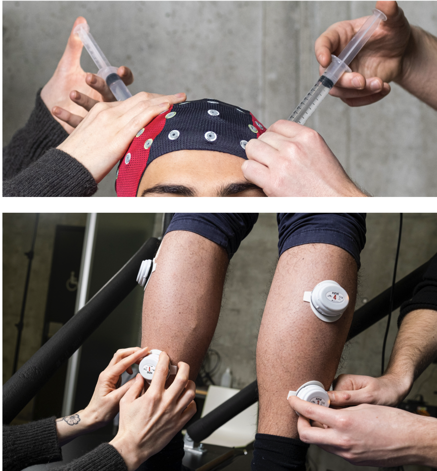
Figure 5.3: BioVRSea Biosignals setup: EEG wet cap and EMG sensors, gastrocnemius lateral, and soleus muscles.
