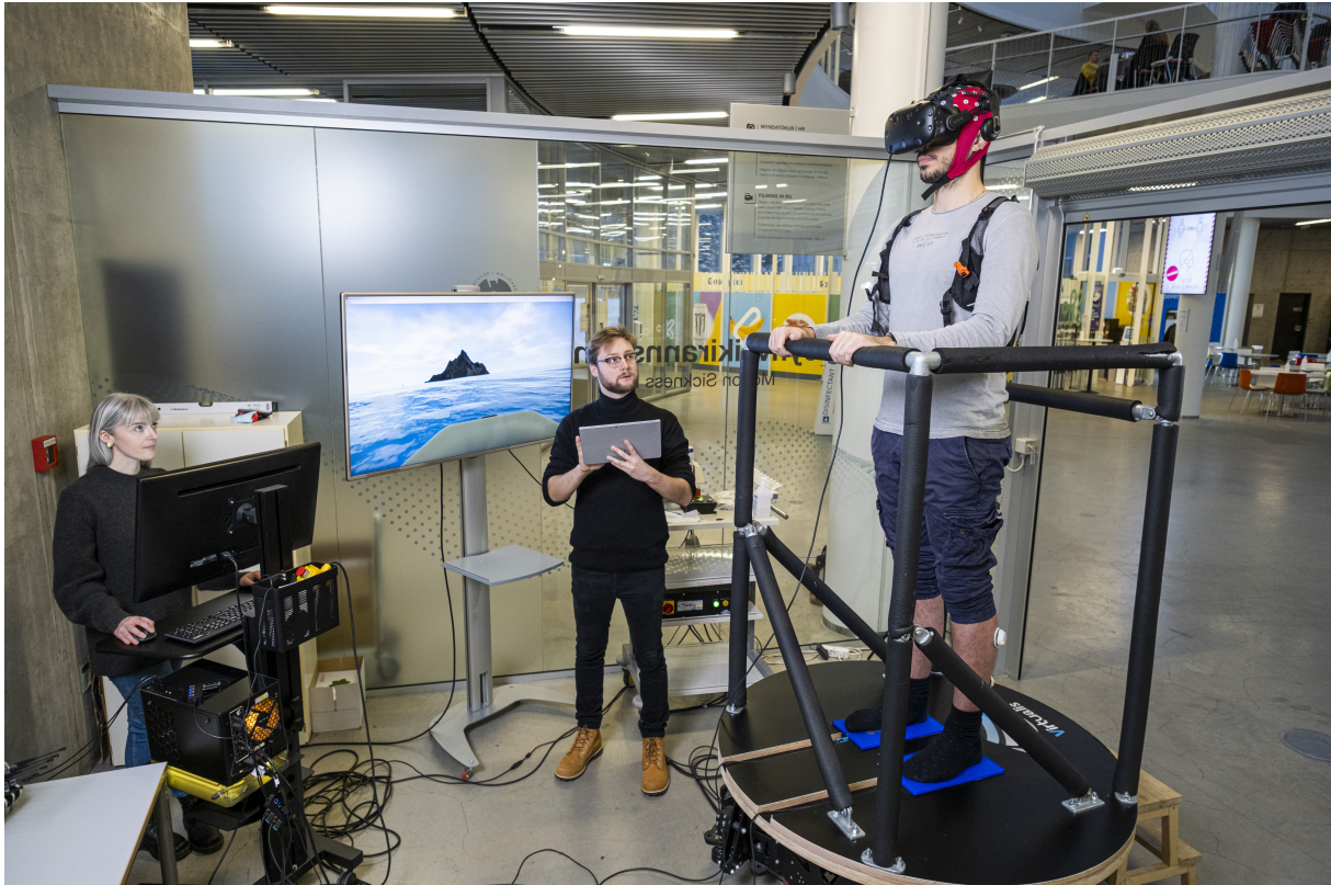
Figure 5.1: A subject on the BioVRSea platform wearing the VR goggles during the sea virtual simulation in the Motion Sickness Lab at Reykjavik University
